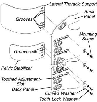
FIGURE 1 - INSTALLING/REMOVING THE LATERAL SUPPORTS
